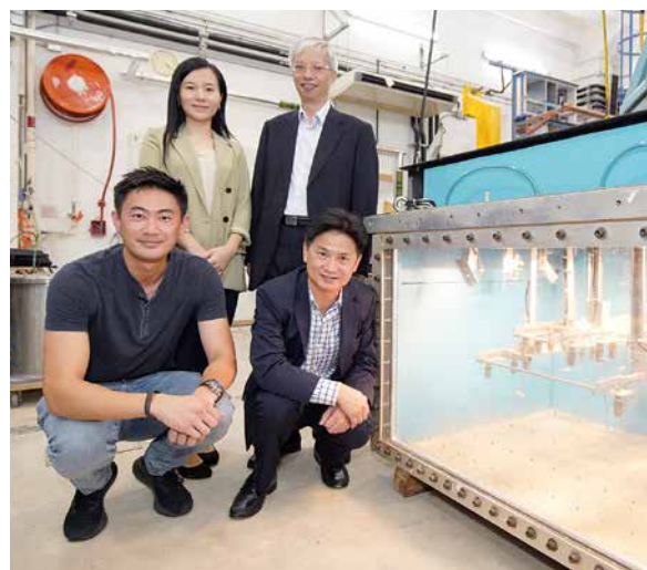
Project members Prof. Charles Ng (front right), Prof. Clarence Choi (front left), Ms. Eva Lam (second row, left) and Ir. W. K. Pun, and HKUST's unique centrifuge environmental chamber developed to simulate effects of extreme weather on slopes.
