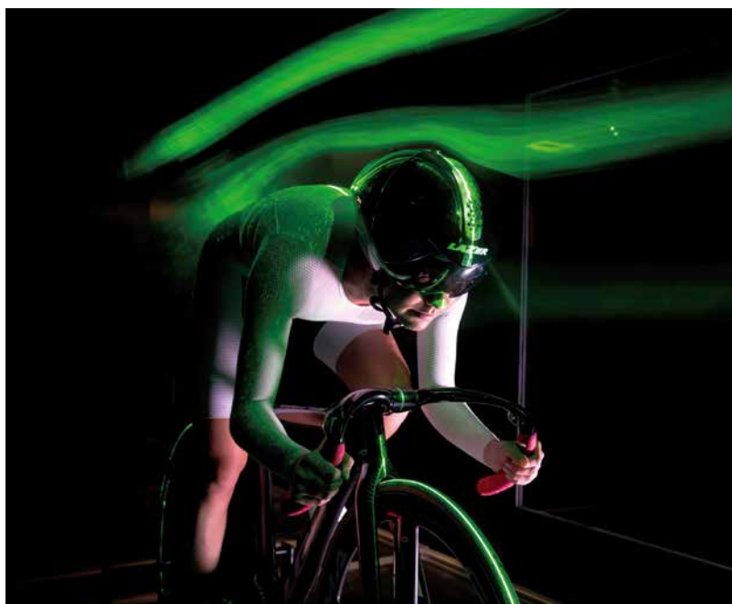
Optimization of riding posture: smoke visualization of an athlete using the aerodynamic test platform.
