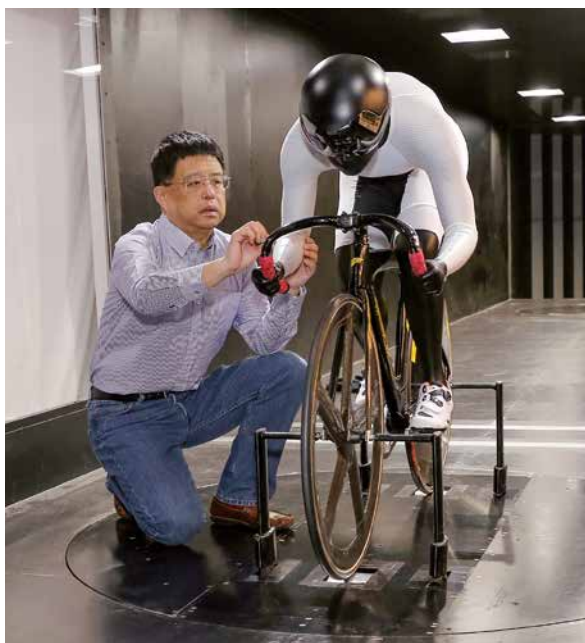
Prof. Zhang Xin prepares to test the aerodynamic design of an athlete's body suit for drag reduction.
