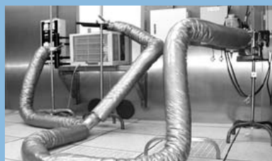
Air-conditioner testing in the Jockey Club Controlled-Environment Test Facility.
