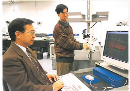
Reversing engineering using contour data obtained from a Coordinate Measurements Machine.
