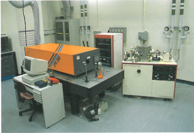
..... The pulsed laser deposition system ready to support photonic materials research.
