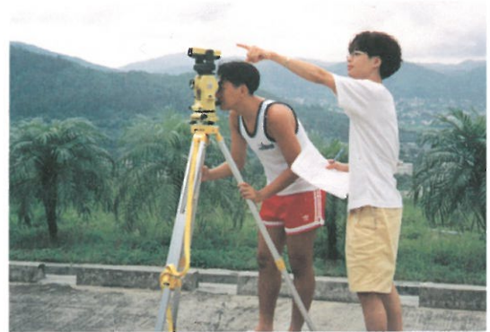
..... Civil & Structural Engineering students practising horizontal distance surveying at the surveying camp.
